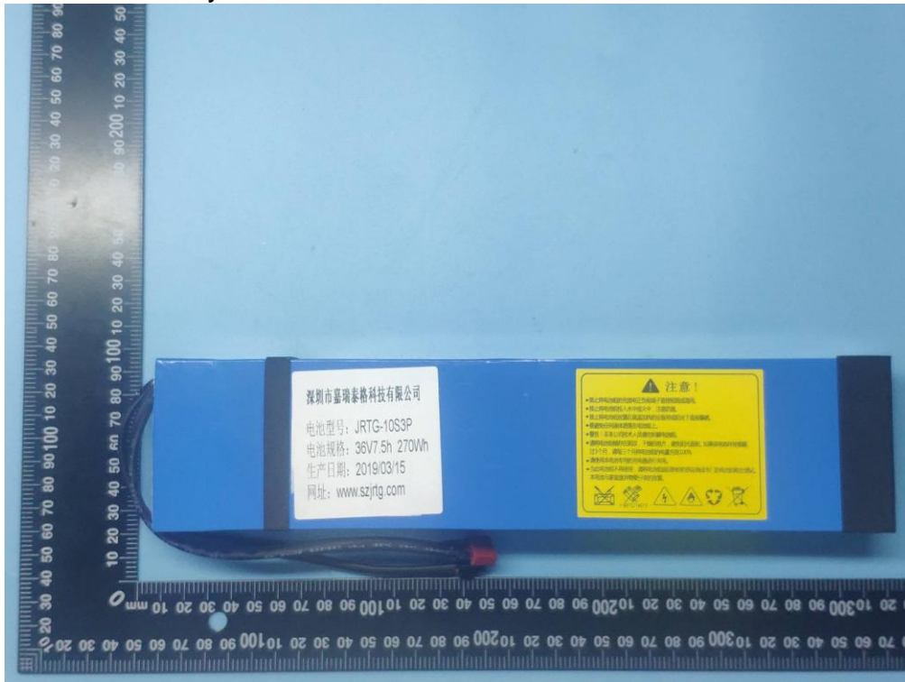
Battery / 电池 (JRTG-10S3P 36V 7.5Ah 270Wh)
