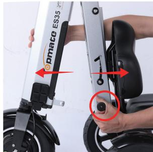
1.Pull the lock buckle outward and unfold the body of the scooter.
