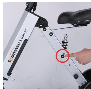
3.Snap the ball into the groove to complete the fixing of the seat cushion.
