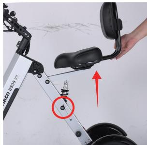
1.Lift the ball upwards to disengage it from the groove.
