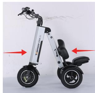
3.Close the vehicle and fasten the buckle to complete the fixing of the vehicle.
