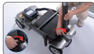
3. There are two angles to choose from. After raising the steering handle and adjust it to a comfortable angle slightly, then tighten the locking bolt. (The locking bolt is located the opposite of the folding limit pin).
