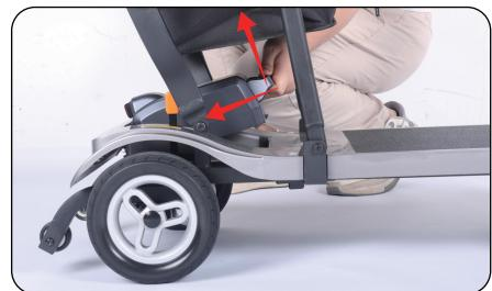
2. Grasp the battery handle, push the battery inward and lift it up ,then the battery will be taken out.
