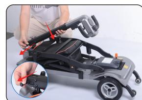
3. Pull the steering handle spring pin, and make the steering handle toward down at the same time, then will lock automatically.
