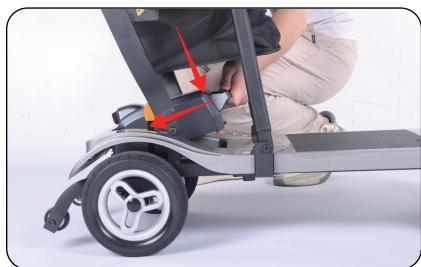
2. Grasp the battery handle and push the battery inward. When the battery is pushed to innermost position, hand leave and the battery will automatically bounce back, then the battery installation done.
