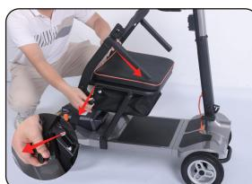
1. Pull the seat limit pin, and push the seat forward to folding down.
