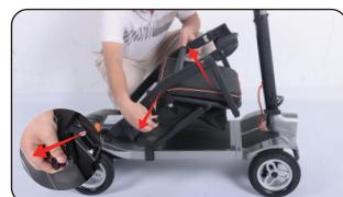
4. Put your hand on the backrest bracket centre beam part, and lift it up until the seat limit pin pops out, at the same time you can hear the "crack" sound, then try to push the seat forward to make sure the seat no longer being folding .
