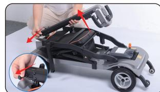
2. Pull the spring pin and make the steering handle stand up at 90° the same time, you can hear the "crack" sound. (Note: If the pin cannot be pulled out easily, try to shake the steering handle up and down before pulling).
