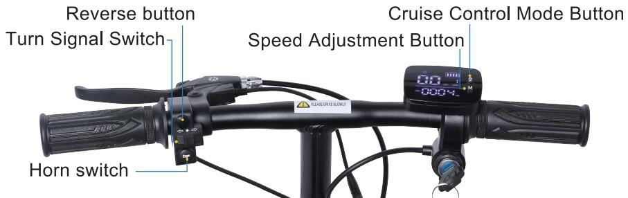
**Activate Cruise Control Mode:** Press and hold the cruise control button, turn the throttle, and release it to activate.
