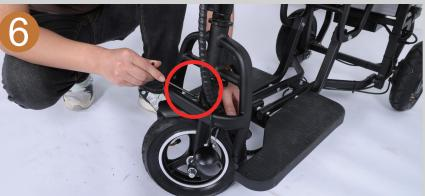
Tighten the screws securely to fix the front mudguard in place.
