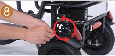
Install the rear fender (tighten screws counterclockwise to secure)
