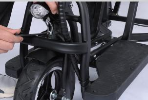
Install the front light and tighten the screws
