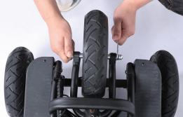
Tighten the screws on both sides to secure the front wheels
